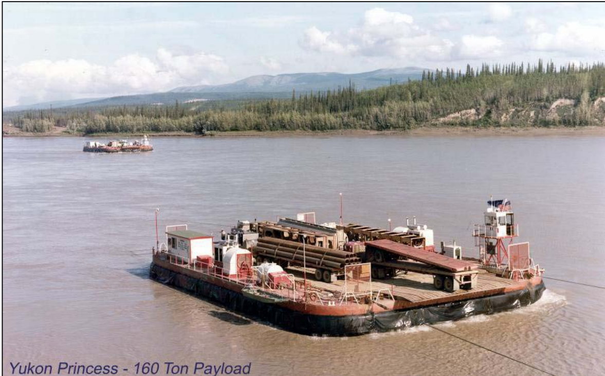
Photo 3 ACB Yukon Princess operating on Yukon River at 5mph showing minimal wake
